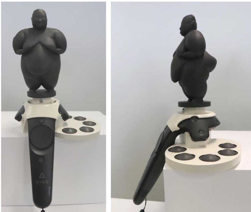
Figure 1: (Top) CAD models of the parts in the support to mount the physical replica over the HTC Vive input controller. (Bottom) Photos of the 3D printed support with the replica of the Female Figurine mounted over the HTC Vive input controller.
